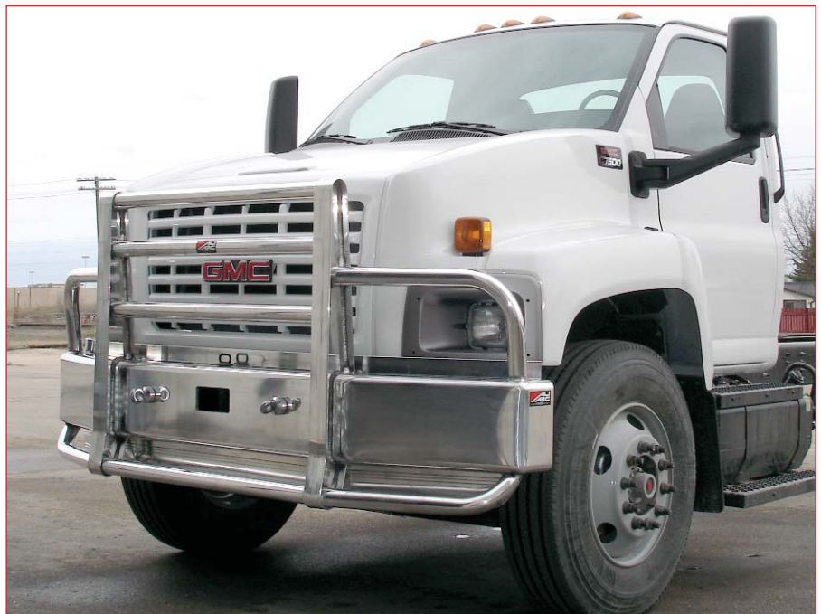
* 1/2" extruded bumper with 2 1/2" tubing & 1/4" wall thickness, integrated tow hitch with easy access tilt system.
